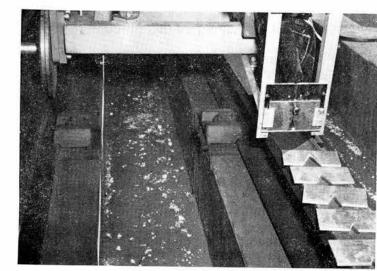
OUTLET plates permit different size beads for different sled speeds.
